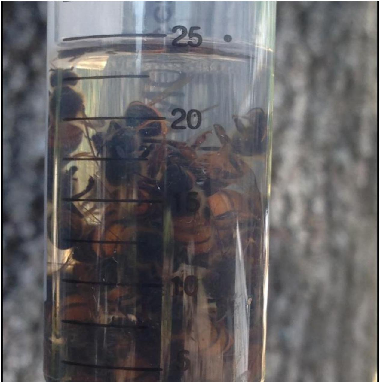
The above photo shows a vial with 30 bees settled to the 20 mL mark. In any case, there should be some free alcohol above the bees. Then seal the lid snugly so that it doesn't leak in transit.
