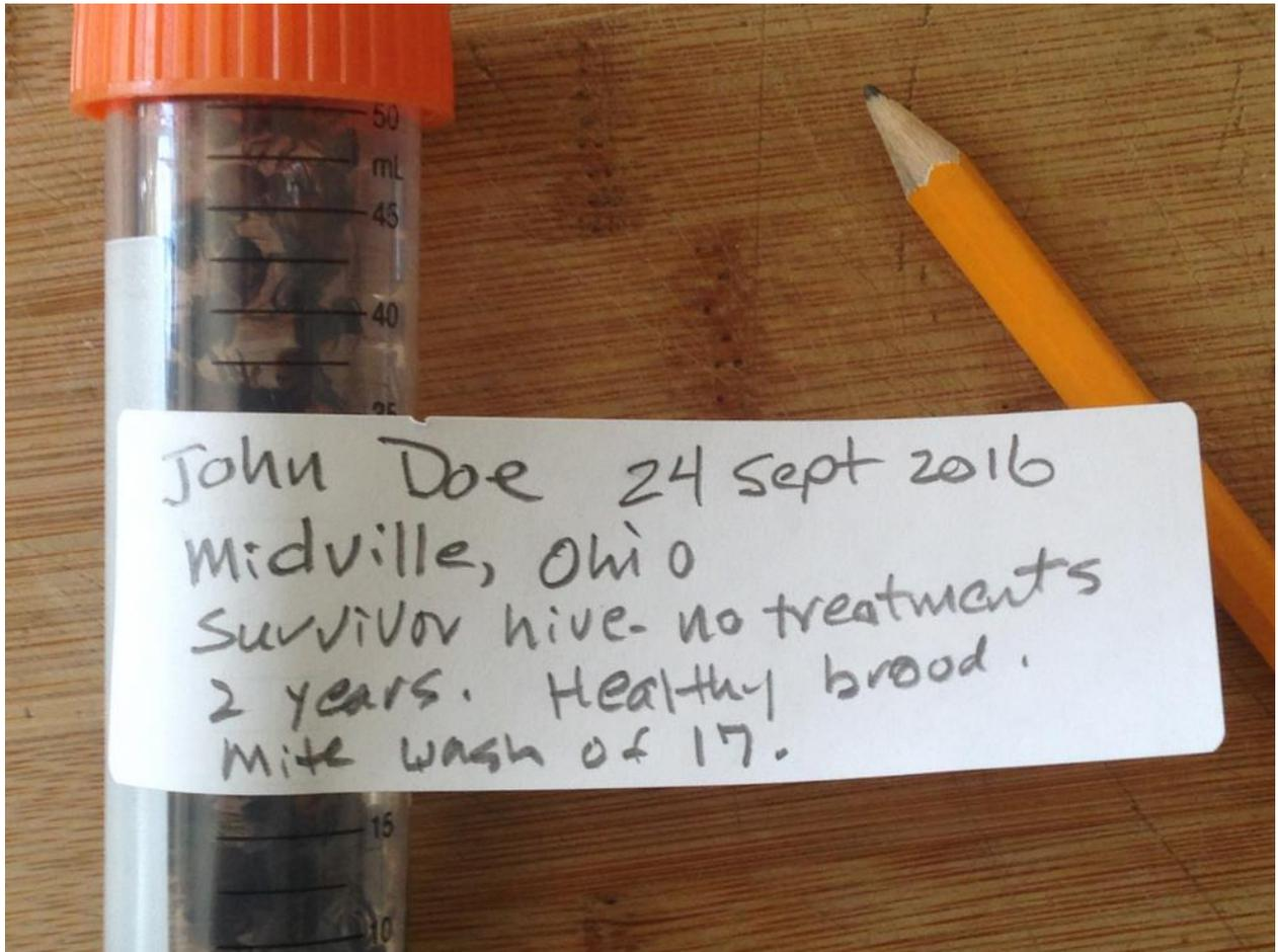
Please label each vial as shown, writing in pencil only (in case of alcohol leakage). Wrap the label around the vial.
